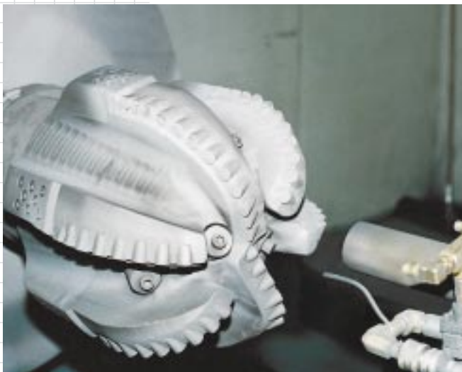
Drill Bits receive an overlay application from Praxair's exclusive detonation gun
