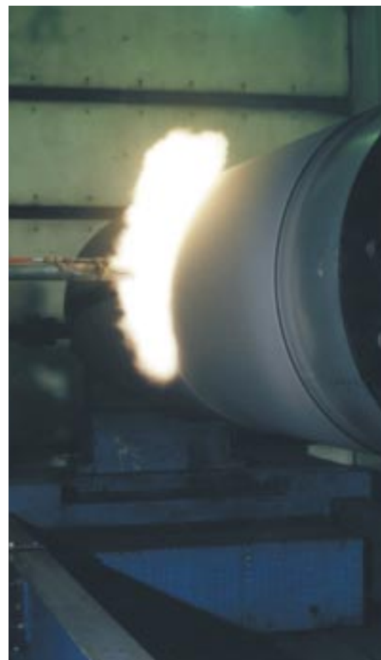
Super D-Gun™ coating of a calender roll
